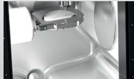
Cleaning-friendly design of the milling chamber and resistant water-repellent coating
